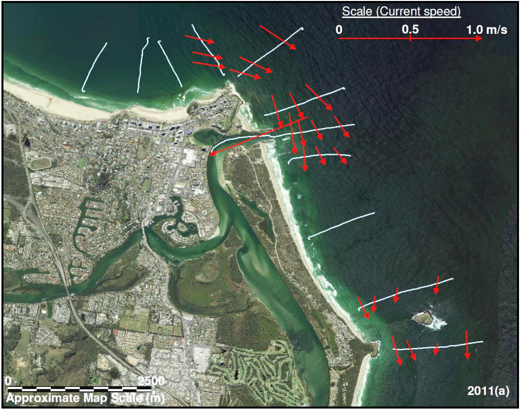
Figure 29: Exercise 3a - Average current velocity vector plot 02/08/2011 (a.m.)
