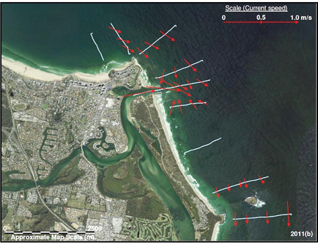
Figure 30: Exercise 3b - Average current velocity vector plot 02/08/2011 (p.m.)
